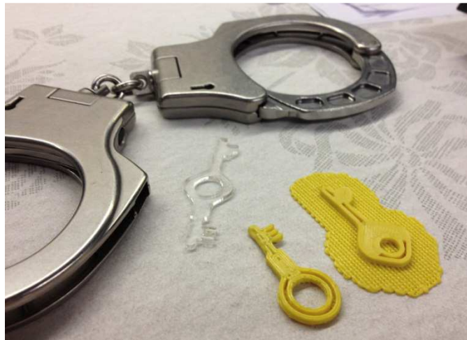
Two 3D-printed and one laser-cut copy of restricted handcuff keys.
